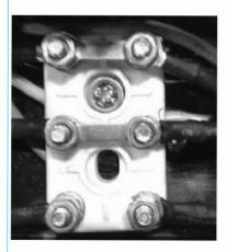
SPECIAL NOTE – The 120v accessory kit is included with this manual. Use the accessories to ensure proper set up using the Wiring Diagram provided on the upper side of the box top. Simply loosen the 220v bridge and reconnect adding the 2<sup>nd</sup> bridge adapter in the configuration listed above & in the Wiring Diagram.
