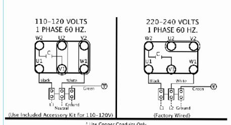
\* Use Copper Conduits Only \* Acceptable for Field Wiring \* Bond Required \* Must be Grounded & Bonded in Accordance with Local and National Electric Codes
